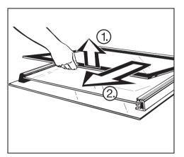
• **Gently** lift the inner pane up and out of the plastic strip.
